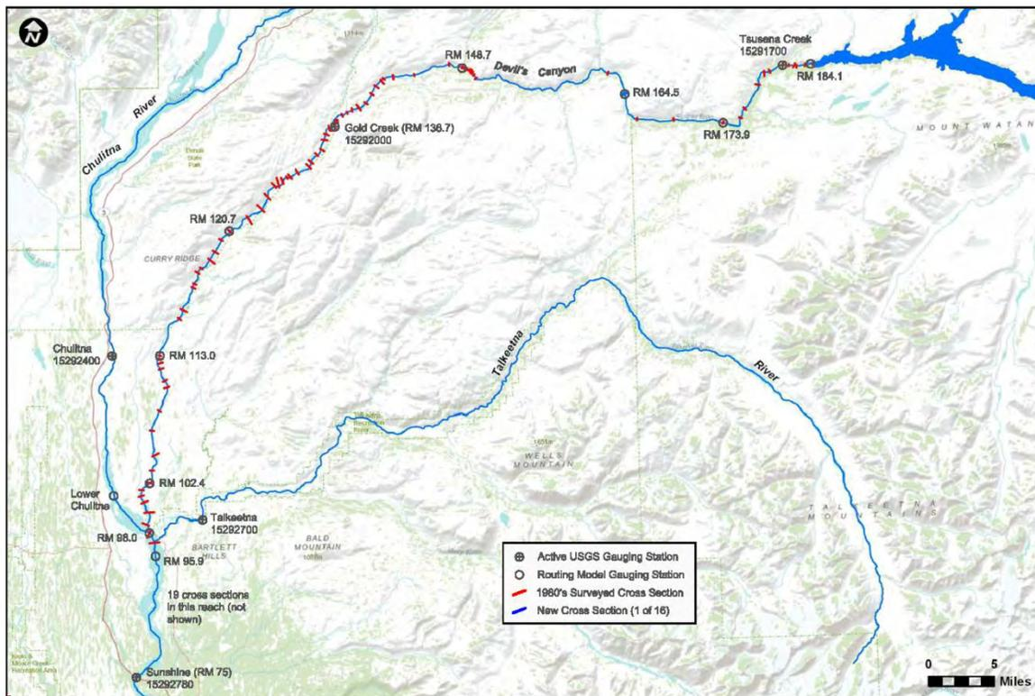
**Figure 2. Study Area, Including Existing USGS Gages, Historic and Potential Cross Sections, and Potential Water Surface Monitoring Stations (note: the Chulitna Gage is inactive)**
