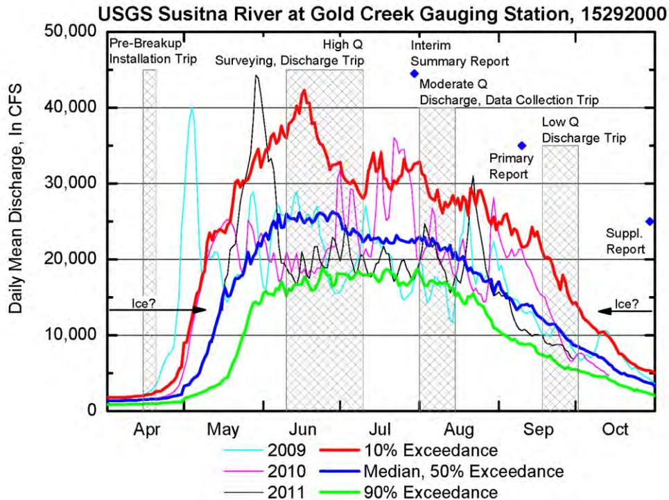
**Figure 3. Project Schedule and Historic Flows at Gold Creek. The August field measurement trip is an optional trip based on flow conditions measured during the first trip and river conditions during August 2012.**
