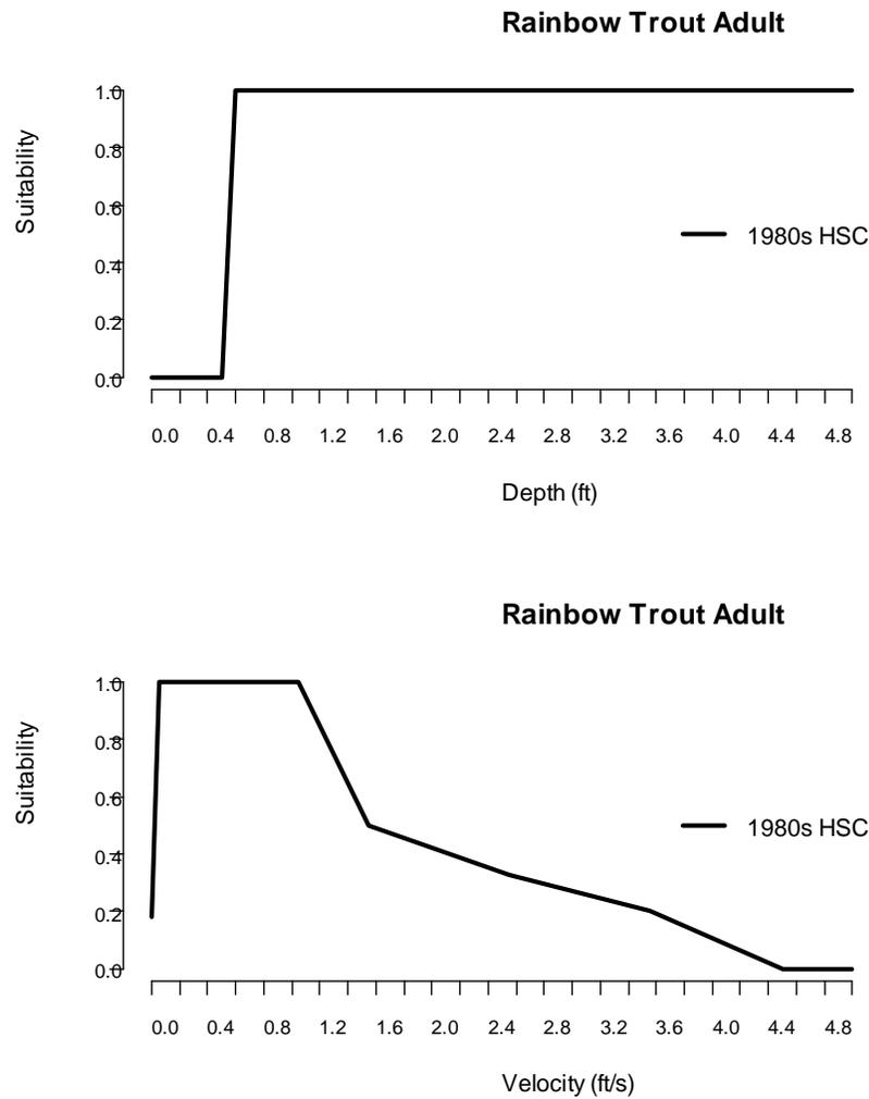
Figure 5-3. Comparison of HSC/HSI developed for Rainbow Trout adult during the 1980s Su-Hydro instream flow studies (Suchanek et al. 1984) for the Middle River Segment of the Susitna River, Alaska and histogram plots generated from 2013-2014 HSC/HSI observations and normalized to the maximum frequency equal to 1.0 for depth (top) and velocity (lower) microhabitat components (2013-2014 HSC database).
